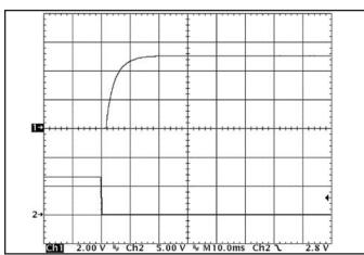
Figure 9: Turn-on transient at full load (resistive load) (10 ms/div).
