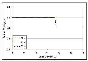
Figure 17: Output voltage vs. load current showing typical current limit curves and converter shutdown points.
