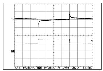
Figure 11: Output voltage response to step-change in load current (50%-75%-50% of Iout(max);  $dI/dt = 0.1A/\mu s$ ). Load cap:  $10\mu F$ ,  $100 \text{ m}\Omega$  ESR tantalum capacitor and 1µF ceramic capacitor. Ch 1: Vout (100mV/div), Ch 2: Iout (5A/div).
