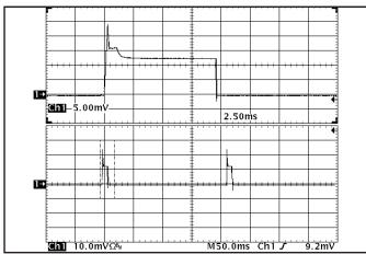
Figure 18: Load current (5A/div) as a function of time when the converter attempts to turn on into a 10 m $\Omega$ short circuit. Top trace (2.5ms/div) is an expansion of the on-time portion of the bottom trace.
